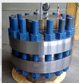
HYDROTEST ON CF ASSEMBLY BLOCK 17 PHASE 2 TOTAL ANGOLA
